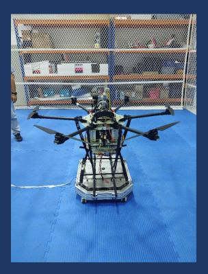
We have successfully flown the drone for a continuous 1.5hrs (without payload) in Feb 2023
