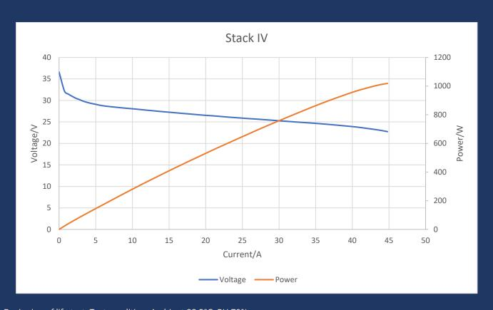
Beginning of life test. Test condition: Ambient 22.5°C, RH 70%
